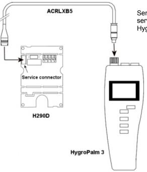
Service cable ACRLXB5 is used to connect the 10-pin service connector of the H290D to probe input 2 of the HygroPalm 3 portable indicator.
